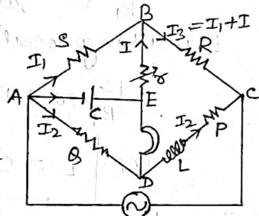
adjusting the resistance in the four arms of the bridge as usual. Next an A.C. Source and a pair of head phones (H.P.) are used and the A.C. balance is obtained by adjusting non-inductive resistance  $\tau$  in series with the capacitor C.
